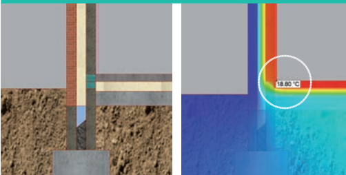
Same Detail with the addition of Almavert – PSI \psi Value = 0.04 W/mK & Minimum Internal Surface Temperature 18.8 °C
