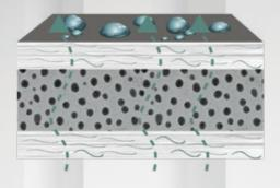
Membrane with **Microporous layer.**Membranes using older microporous technology are more suspectable to UV damage, delamination, and ageing. The layer is stretched with calcium carbonate added during production which creates holes in the material. Their waterproof performance and claimed breathability can be easily affected during installation. This layer utilizes physical vapor transport pores which can easily be blocked.
