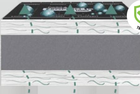
TPE Monolithic film guarantees **breathability**, thanks to a non-physical, absorption and diffusion reaction, rather than a micro perforation process as seen in microporous products. This means the layer is **continuous, dense and free of pores**, offering a complete long-term barrier against the passage of water, while achieving increased durability.
