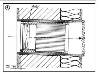
Connect cables to plugs, insert pin and socket connectors into the recess of the heat exchanger casing.
