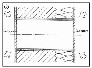
Remove the plaster protection cap outdoors. Assemble the outer grille using the integrated claw fasteners (tighten screws).
