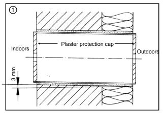
Apply plaster indoors and outdoors. If outer closure is plastered, first replace the plaster protection cap outdoors by an outdoor closure piece.
